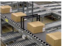
Two different models are available: high resolution (AS1-HR) or standard resolution (AS1-SR). In the first case the light array has 16 beams, while in the second case the beams are reduced to 6. In the AS1-HR model, the selection inputs of the SCAN MODE, can configure 4 different crossed-beam scanning modes. These different modes allow to vary the detection performances, in particular the resolution can be increased to 0.2mm thickness, or the response time up to less than 3ms.
